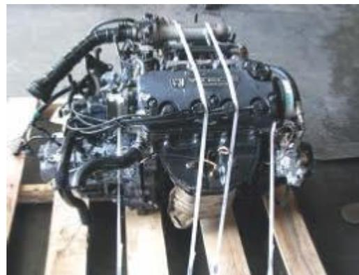
Plastic band strapped engine. 4 plastic straps done by machine and tight. Engine sits flat on pallet, no tyre needed. Ideally should be sat on rags/mat, but not needed as engine is drained, and is very clean. Straps could benefit from protection, but if bands touch smooth areas then are ok.
