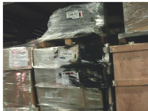
good and bad examples of palletised engines for guidance. Should always be drained of fluids.
